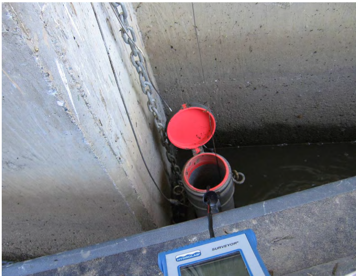
Figure 5.3-1 Downloading data from a Hydrolab MiniSonde5, located within its protective casing, using a Surveyor4a, at the Highway 97 Bridge.
