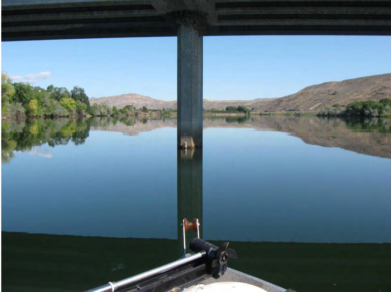
Figure 5.1-1 Water quality monitoring instrument housing mounted on the downriver side of a Monse Bridge piling.
