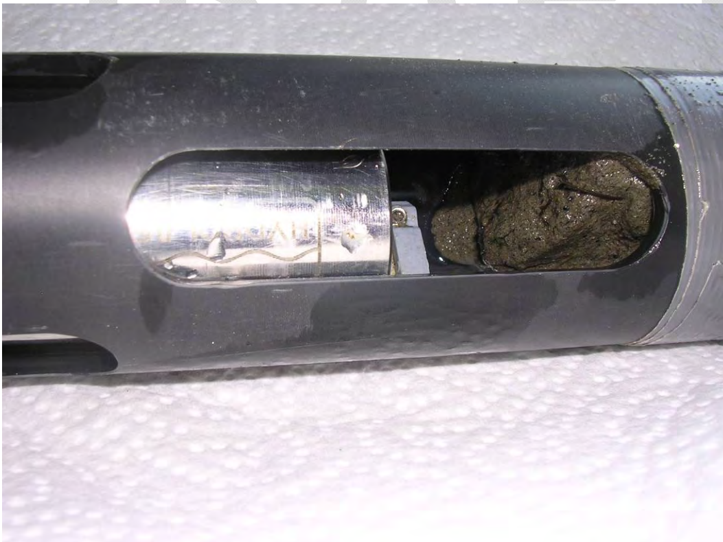
Figure 3. Water quality probe after collection from Monse on the Okanogan River, 2009.
