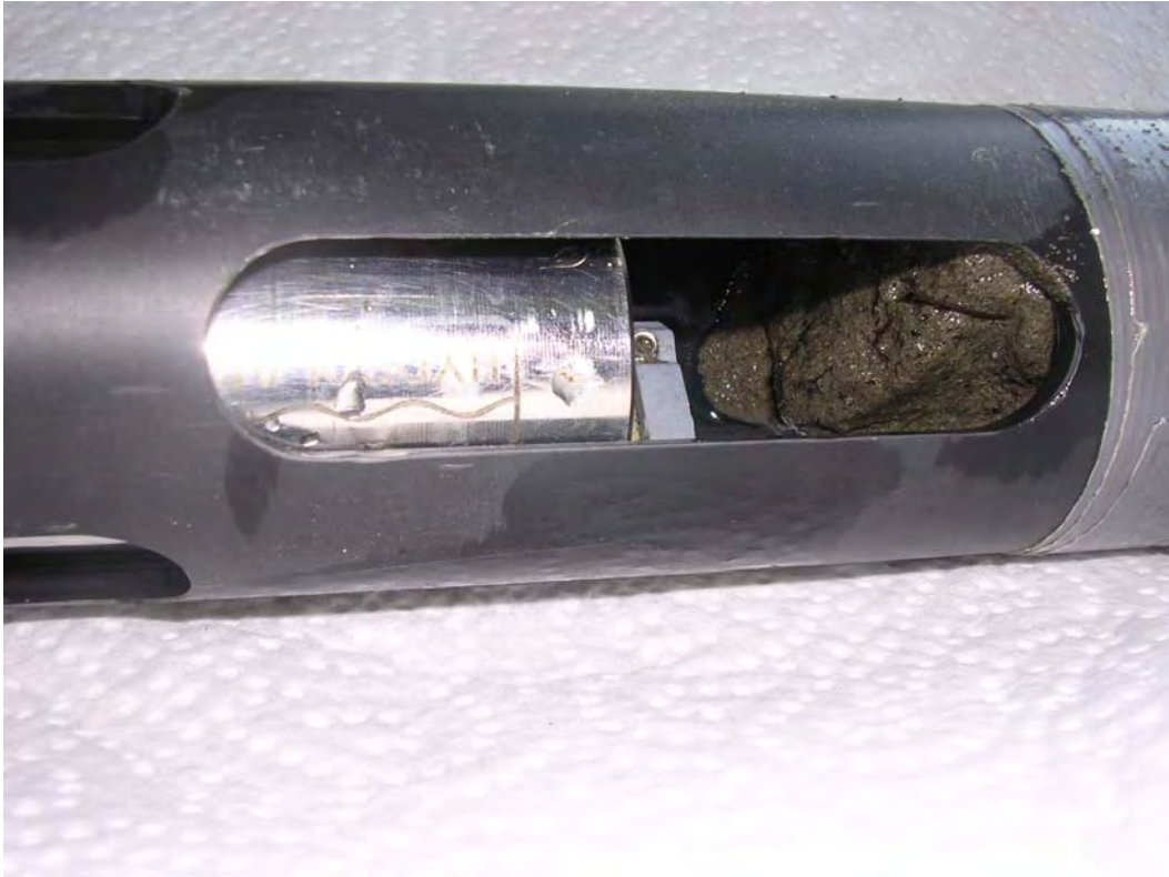
Figure 2. Hydrolab and sediment blockage after retrieval from Monse on the Okanogan River, 2009.
