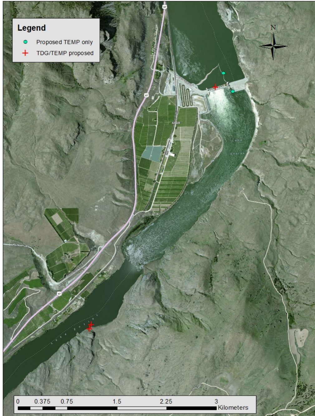
Figure 3. Proposed locations of forebay and tailrace TDG/temperature stations and temperature stations only. Sensors pictured include two redundant tailrace TDG stations and one forebay station above turbine unit six, one fishway temperature and auxiliary water supply station and one forebay water temperature profile sensor (surface, mid and deep depths) affixed to the debris boom.
