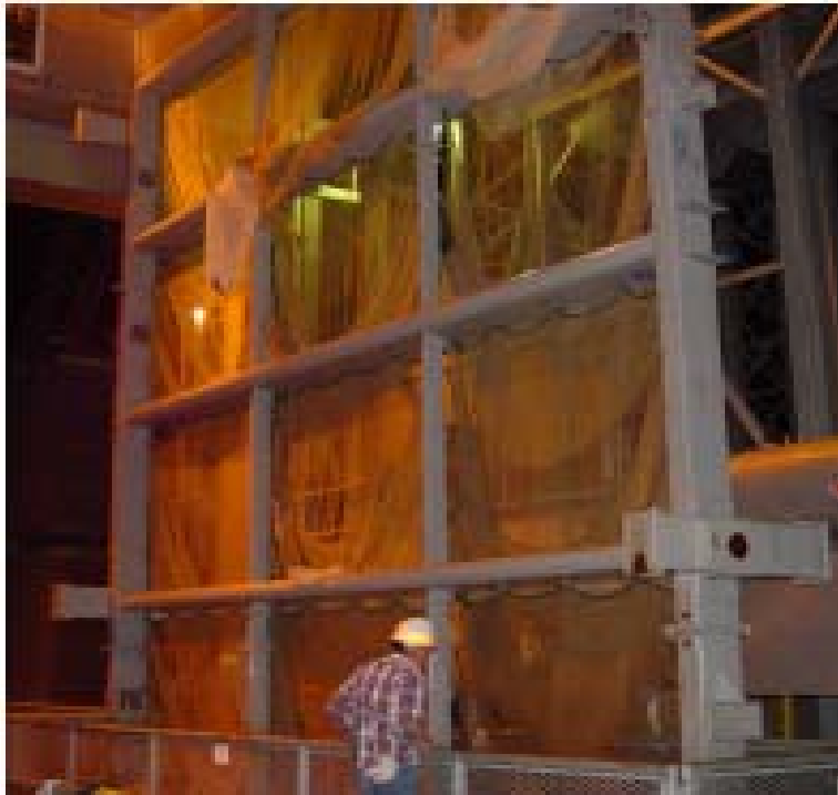
Figure 17. Fyke net removed from a turbine gatewell at John Day Dam (Moursund et al. 2003).
