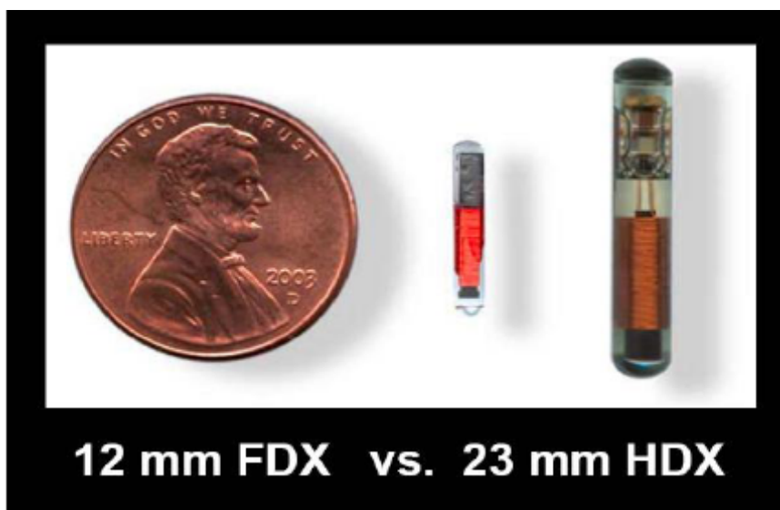
Figure 5. Full duplex (left) and half- duplex PIT-tags (Cummings 2007).
