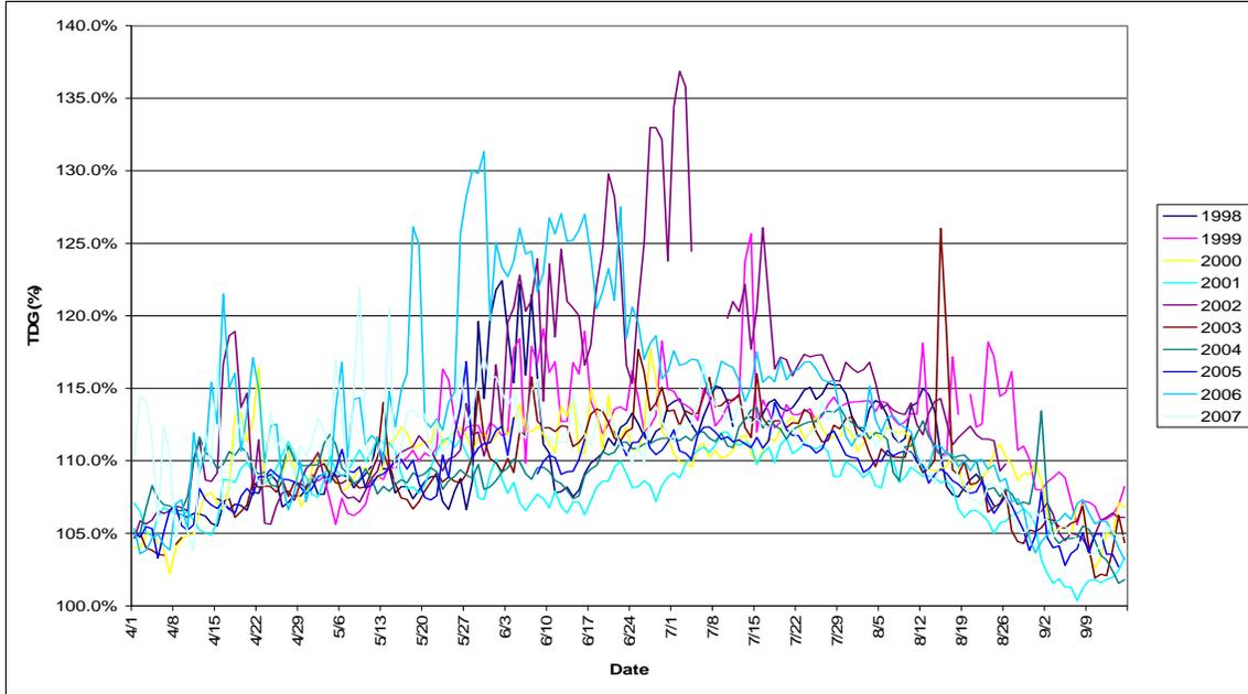
**Figure 2.2-2 Wells Dam tailrace average 12-hour high TDG measurements. The average 12-hour high is defined as the average of the 12 highest hourly readings within a 24 hour period. Monitoring season is typically April 1 to September 15. Data for years 1998-2007 (Breaks in data are the result of equipment malfunction).**
