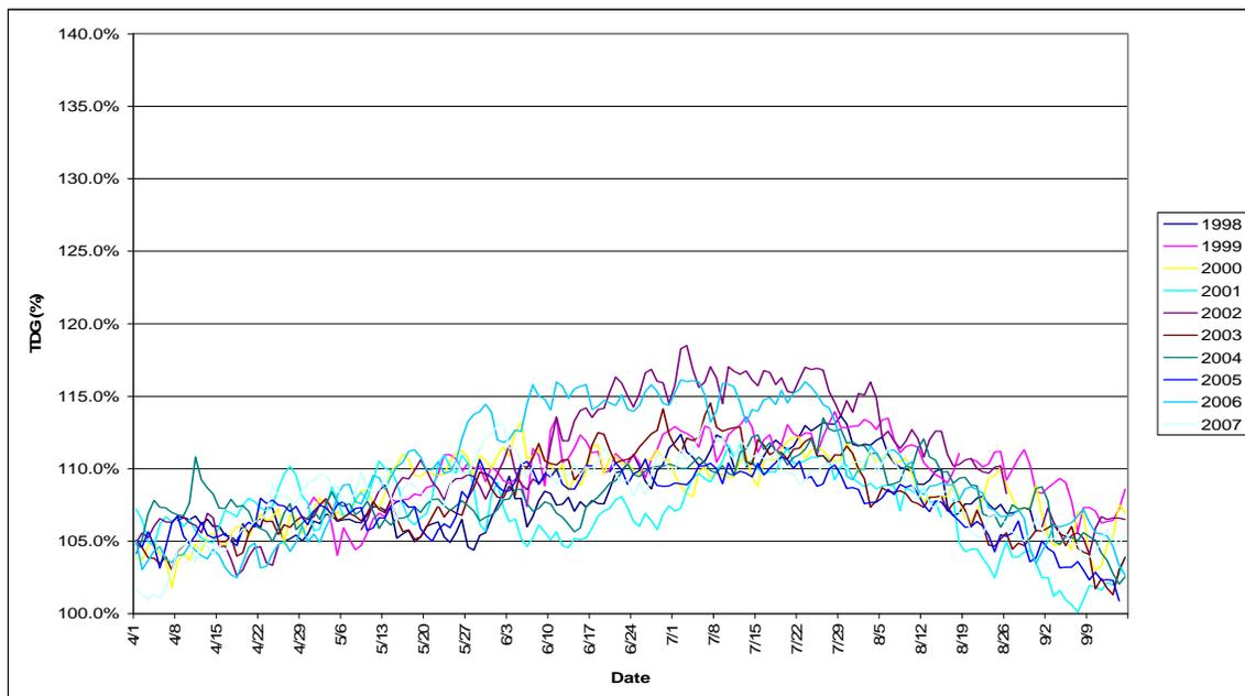
**Figure 2.2-1 Wells Dam forebay average 12-hour high TDG measurements. The average 12-hour high is defined as the average of the 12 highest hourly readings within a 24-hour period. Monitoring season is typically April 1 to September 15. Data for years 1998-2007.**
