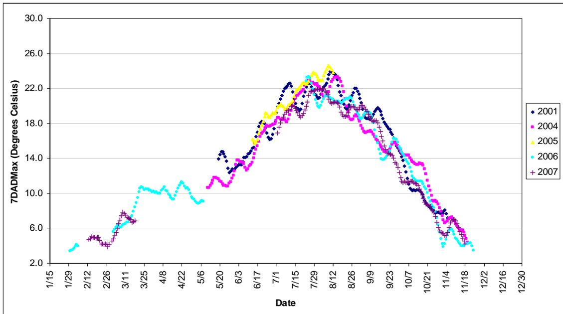
**Figure 2.2-5** 7-DADMax water temperature collected in the Methow River upstream from the influence of Wells Dam (RM 1.4) using Onset temperature loggers for years 2001-2007. Data were unavailable in 2002 and 2003.
