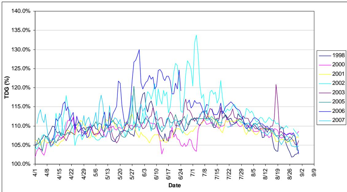
**Figure 2.2-3 Rocky Reach forebay average 12-hour high TDG measurements. The average 12-hour high is defined as the average of the 12 highest hourly readings within a 24 hour period. Monitoring season is typically April 1 to August 31. Data for years 1998-2007 (Breaks in data are the result of equipment malfunction).**
