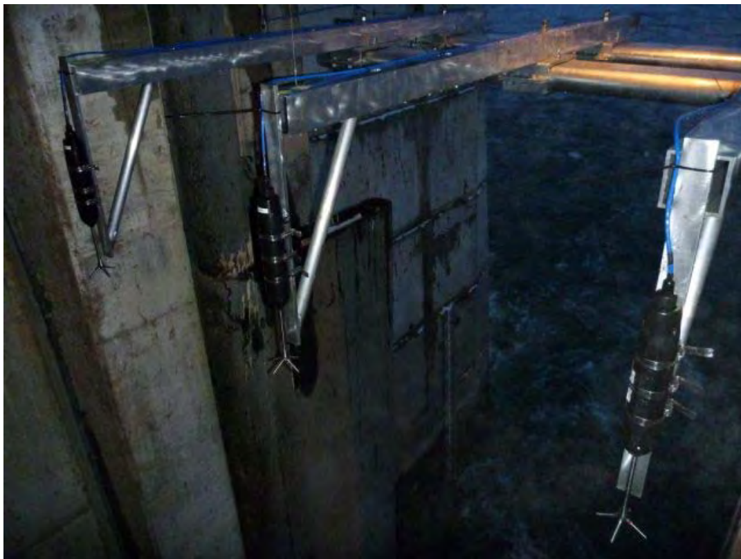
Photo 4: ADVs shown mounted on the support arms prior to being lowered into the water for testing. (Photo by Douglas PUD)
