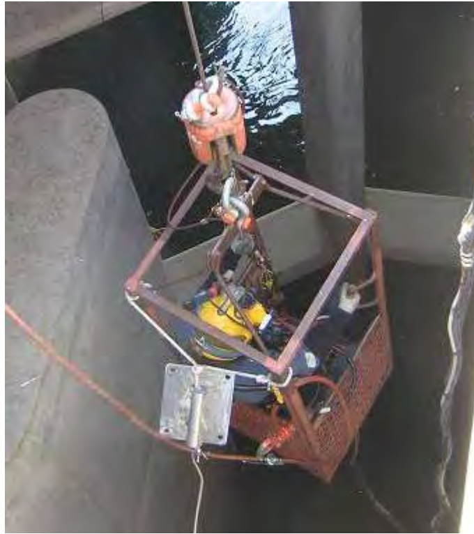
Figure 1. Diver being lowered into the west side fish ladder prior to deployment of the DIDSON. Also shown is an aluminum plate with a pipe attached hanging from the man basket. This plate was mounted on the wall adjacent to the ladder entrance; another plate (not shown), with the DIDSON attached to it, was then fastened to the pipe.
