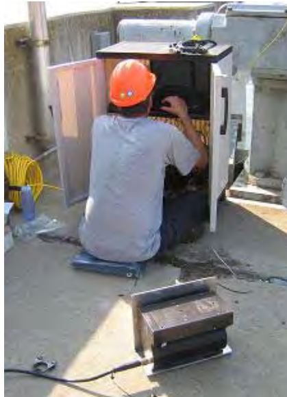
Figure 5. Cabinet used to house the electronics for the DIDSON system at the west side fish ladder. The DIDSON sonar is shown in the foreground attached to an aluminum bracket.
