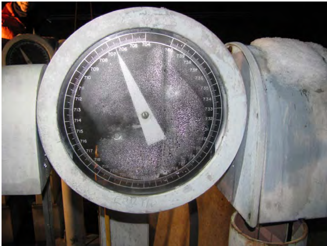
Photo 6: Tailwater gage used to record the tailwater level. The Collection Chamber gage is in the background to the left. The difference between these two readings indicates the head drop across the fishway entrance. (Photo by NHC)
