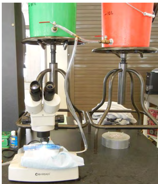
Figure 1. GBT examination station used at Rocky Reach juvenile bypass facility to examine juvenile salmonids exposed to high TDG concentrations.
